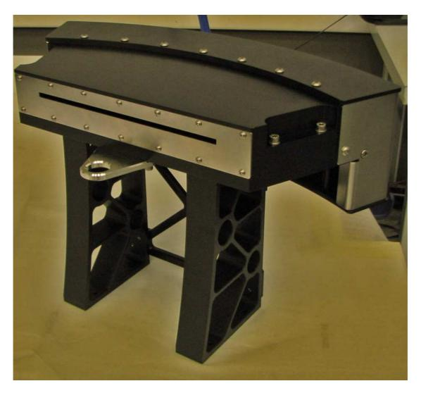
Figure 1. The fast position sensitive strip-detector (SLS Mythen 2 design) of BL04-MSPD.
